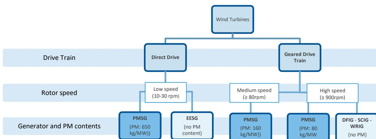
Figure 8: Wind Turbine Configuration and Permanent Magnets (PM) Content (Source: Pavel et al. 2017a)
